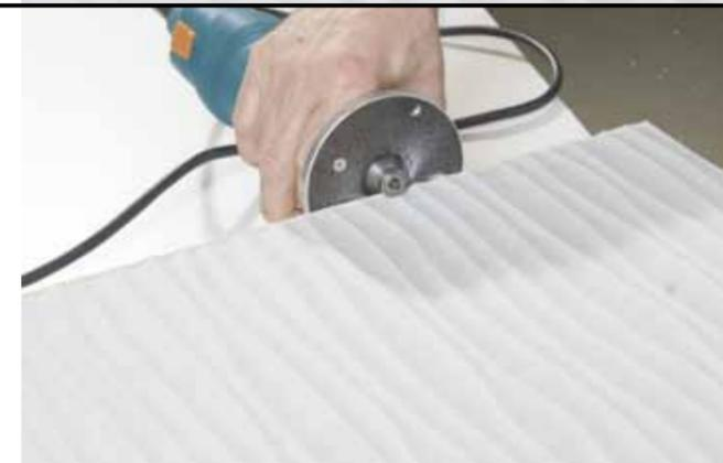
Refinish the excess length with a profile cutter. Use primarily small tool profiles. A ball bearing guide ensures a smooth tool guidance.
