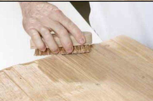
Finally clean structure oriented with a fine copper wire brush.
