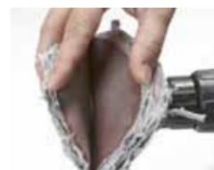
Finally clean structure oriented with a sanding pad (ap. grain 100).
