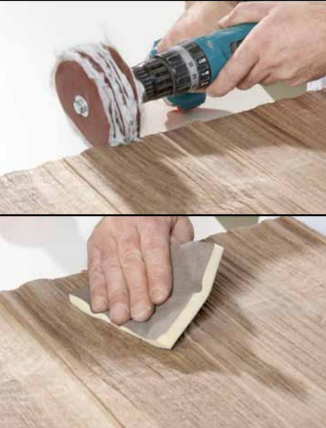
Spalt linear boards don't really need edge banding however it is feasible (see page 4). After cutting for crushing and trimming the edge - here is how we do it: Mount 10 to 15 layers of sand paper face to face separated by washers on a thread bar and secure it with a nut at the end. Powered by a drill or cordless screwdriver this tool simplifies your finishing of our Spalt surfaces.
