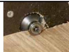
Refinish the excess length with a profile cutter. Use primarily small tool profiles. A ball bearing guide ensures a smooth tool guidance.
