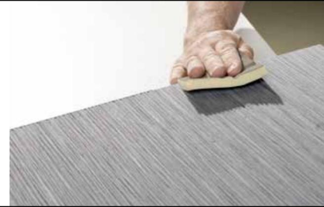
Finally clean structure oriented with a fine copper wire brush.
